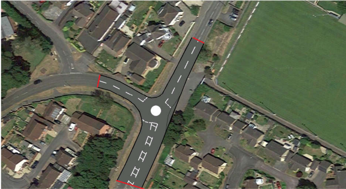
Figure 22 – Example of mini roundabout at junction of Silver Street and Meadow Park
